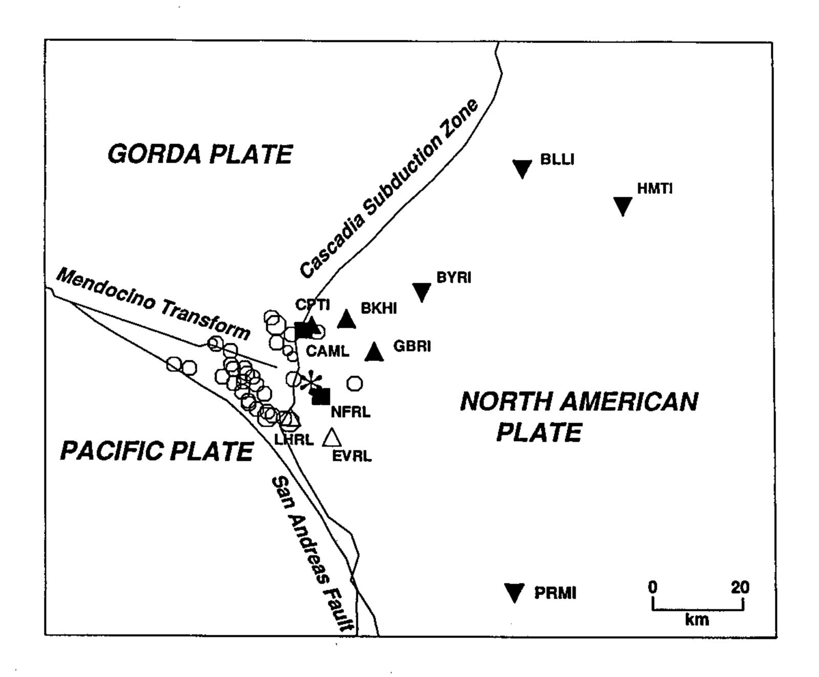
Figure 1 Location of all M>3.0 aftershocks (open circles) in Cape Mendocino aftershock data release 1. Solid symbols show the locations of stations with broadband sensors where the upright triangles, upside down triangles and boxes indicate Guralp CMG-3, STS-2, and Kinemetrics SH-1 and SV-1 sensors respectively. The star marks the mainshock location.
