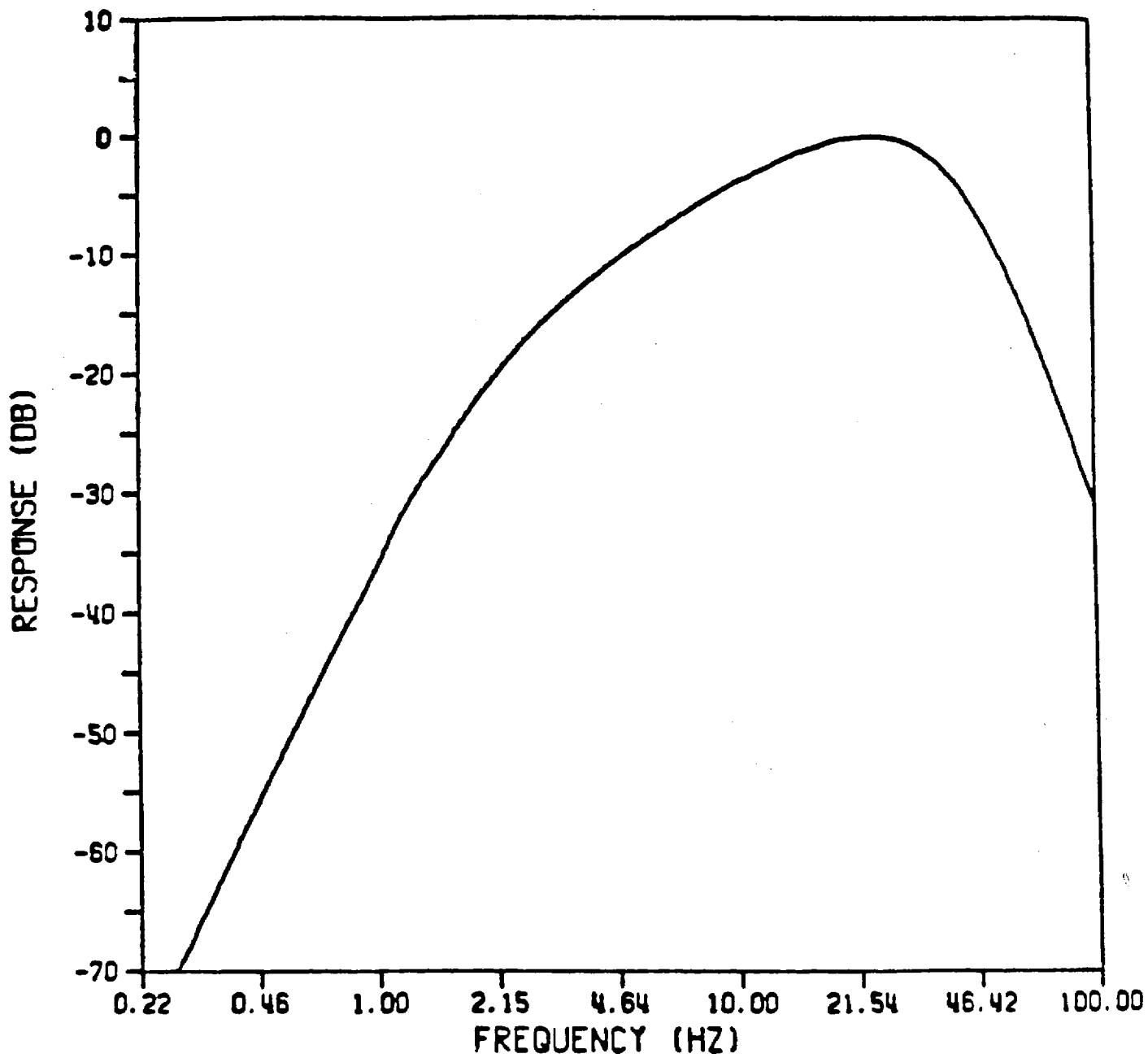
Figure 2 .--System Response Curve for Seismic Recording Units.
