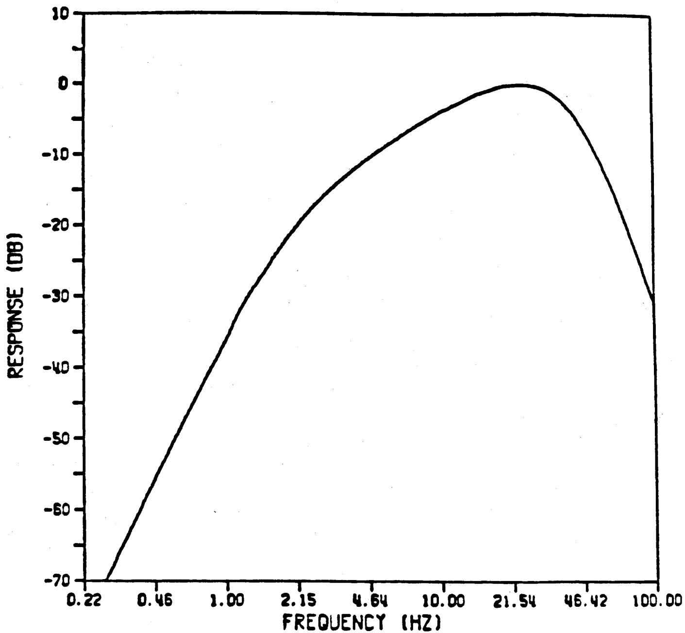
Figure 17: System Response Curve for cassette recording units with 2-Hz seismometers.
