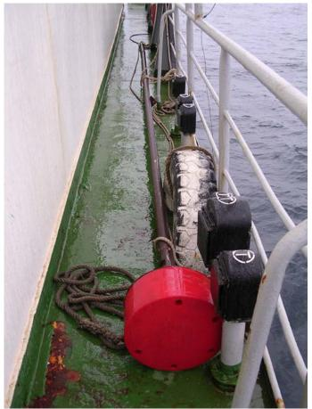
Figure 1: Echosounder with its pole
