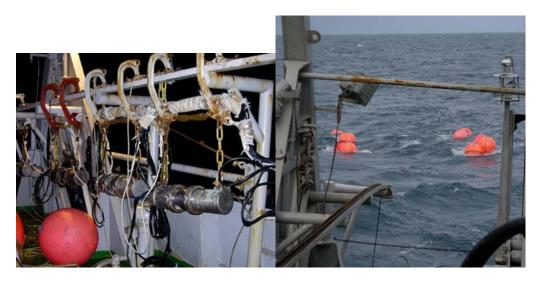
Figure 2: Port airgun string (left) and deployed airgun source (right)
