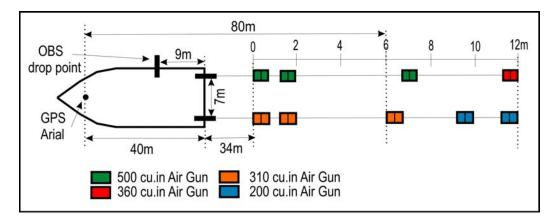
Figure 3: Geometry of airgun array. Guns were towed at ~9 m depth
