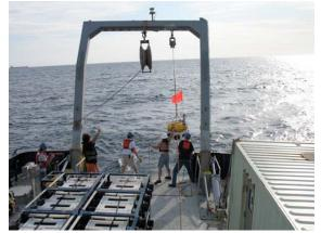
Retrieving the first part of the tethered instrument using the A-frame.
