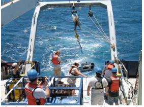
After feeding out most of the 400 m of line, the anchor and acoustic release package was deployed.
