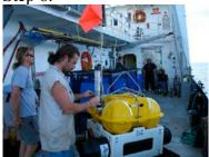
Secure the radio, strobe light and red flag, make sure the radio and strobe are working properly.
