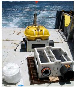
Tethered OBS setup, the float is attached to a frame containing the data logger and will be suspended 400 m above a second frame containing the acoustic release attached to the anchor. We used 400m of polypro neutral buoyancy rope.
