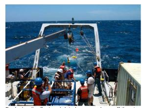
Deploying the float and data logger package off the stern using the crane under the A-frame.
