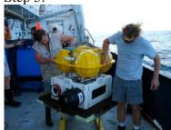
Attach float package to the top of the frame.
