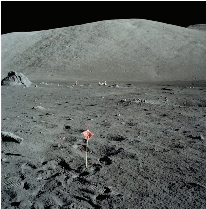
Figure 8. One of the geophones depicted in Figure 7 "planted" at the Apollo 17 landing site.
