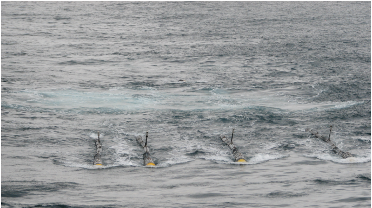
Figure 2. Linear air gun arrays shown onboard and towed behind the vessel. The arrays were spaced 6 m apart and totaled 40 guns of which 36 were active for a total of 6600 cu. in.
