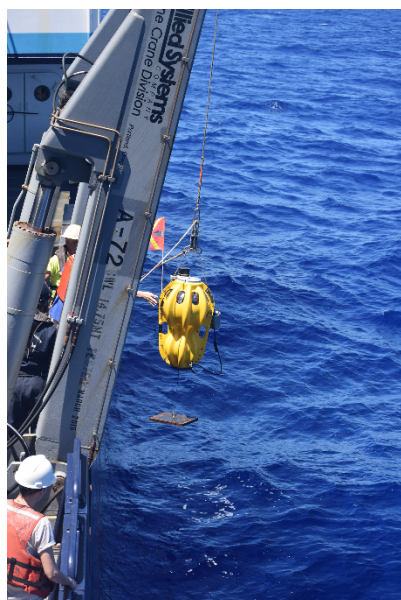
Figure 7. OBS deployment using the starboard A-frame.
