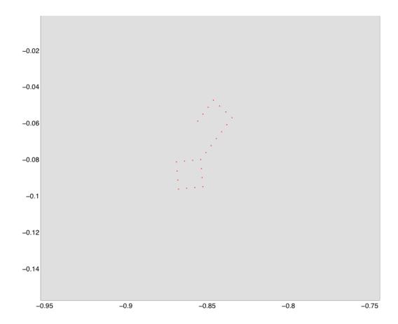
**Figure 2**: Detailed geometry of the array. Geophone positions are shown by red dots. Map axes are in kilometers following the orientation of Figure 1.
