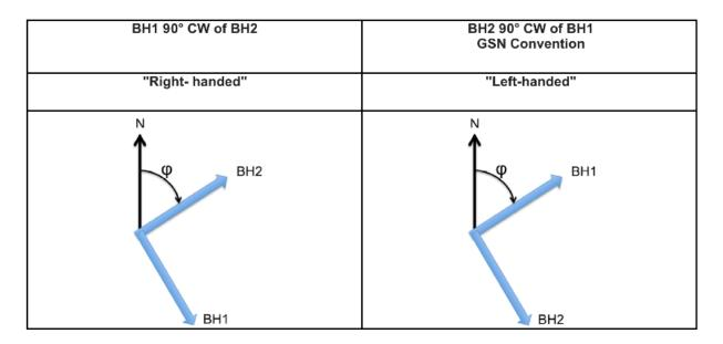
Because OBSIP instruments are built and operated by three different IIC's, the usage of default relative horizontal orientation of channels varied in Year 1. In Year 2, all of the data was intended to be uploaded in the GSN convention (BH2 90° CW of BH1). The Cascadia data has been corrected for both Year 1 and Year 2 so that all data follows the GSN convention (BH2 90° CW of BH1).
