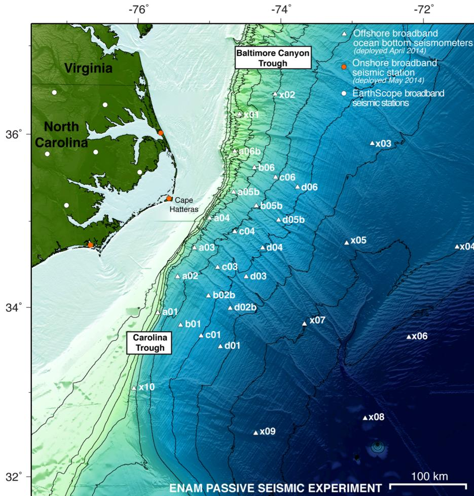
**Figure 1:** ENAM Broadband seismic component. White triangles represent the thirty WHOI broadband OBS and the orange circles are the three onshore broadband seismometers installed on the outer banks.
