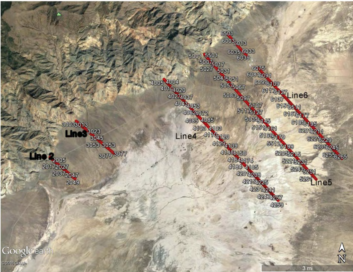
Figure 2: Google Earth images showing orientation of the five seismic profiles along which ambient noise was acquired. The numbers shown are station numbers. They have a spacing of about 64 m for Lines 2, 3, 5 and 6 and 34 m for Line 4.
