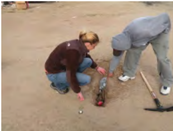
Figure 5. (A) Typical installation of a geophone, provided by IRIS, to be used in the Dixie Valley Geothermal Wellfield new ANS project. (B) Texan digitizer whose size is 3-inches in diameter by 7.7-inches long. (C) The geophone and digitizer is deployed a few inches below the ground surface and covered with soil. Note that the digitizer is covered by a clear plastic bag and taped closed.
