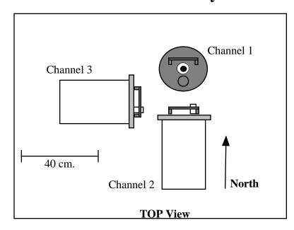
Channel Order (positive voltage on DAS channel means ground moved in given direction)
