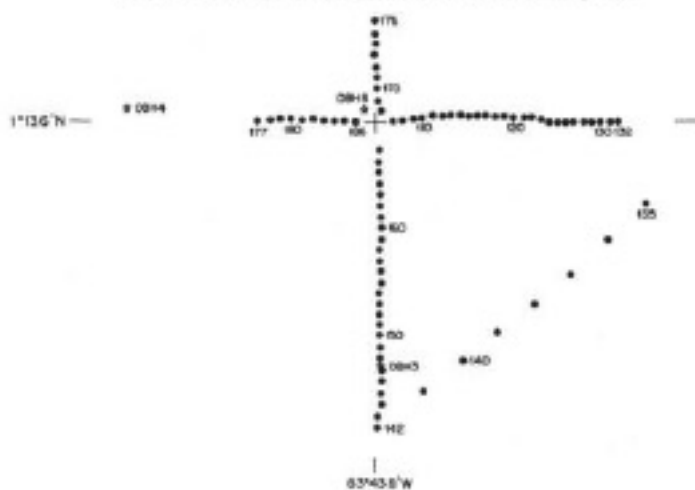
B. Shot locations for geophone at 4200 meters below rig floor
