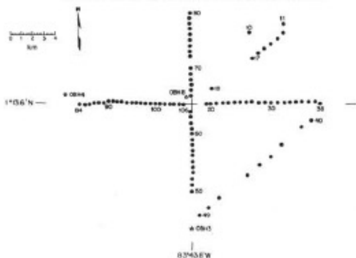
A. Shot locations for geophone at 3800 meters below rig floor
