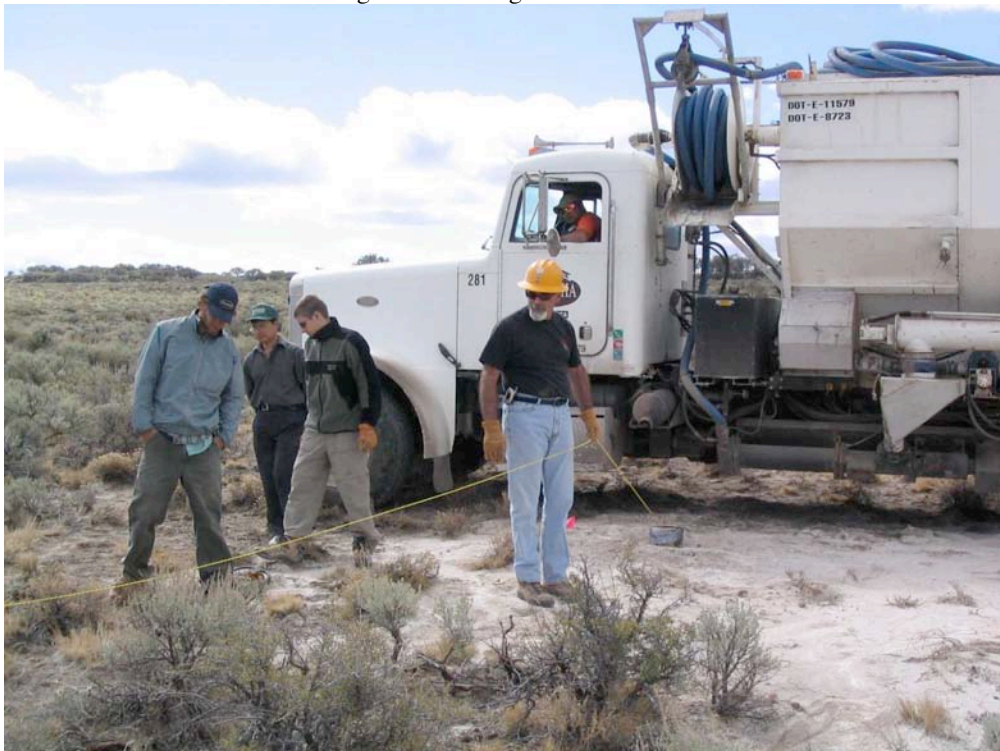
Figure 2. Tom Burdette lowering boosters strung on detonation cord down the hole at SP1, explosives delivery truck in the background.
