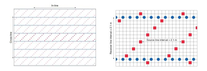
**Figure 1**: Acquisition swath and patch for the 3-D experiment. The red squares represent the sources and the blue circles represent the receivers. Six receiver lines were active for each shot line. Except for rolling in and rolling out at the northern and southern ends of the seismic array, all shot lines were recorded by 3 receiver lines to the north and 3 receiver lines to the south, giving a total of 630 (maximum) channels.
