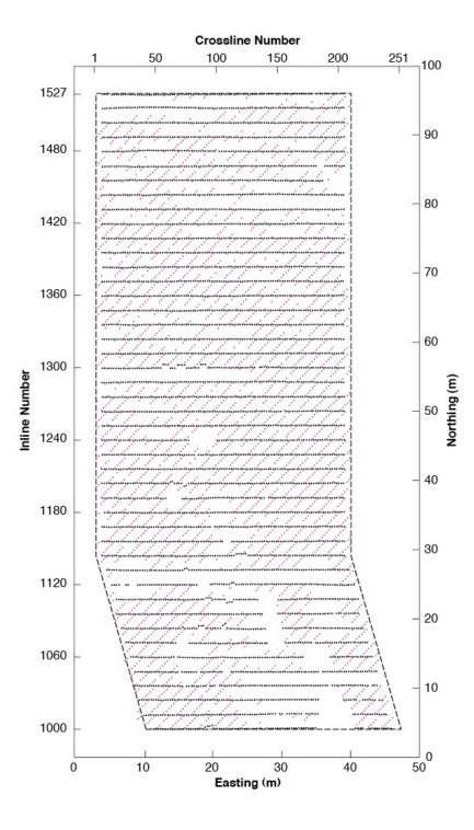
**Figure 2**: Acquisition layout for the 3-D experiment. The black dots represent the receiver lines and the red dots represent the source points. The inline and crossline numbering is consistent with the one presently in the data trace headers. Northing and Easting are relative to the southwestern corner of the survey area for display purpose only. The data tracer headers contain the absolute coordinates. The white areas are gaps in the acquisition.
