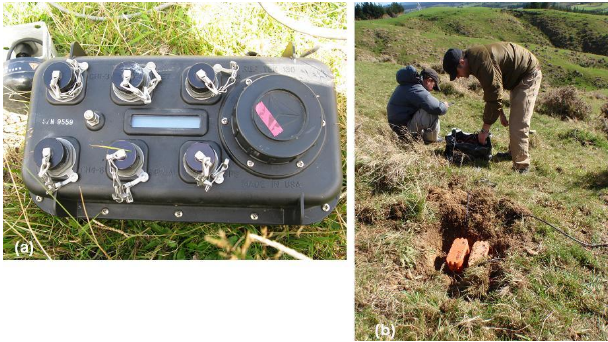
Figure 3.2 (a) REFTEK RT130 (b) 3 component sensors (3C) attached to RT130 collocated with the 3C sensor connected to 3 single Texan instruments.
