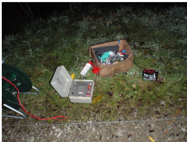
Figure 4.1 Shot firing trigger system.
