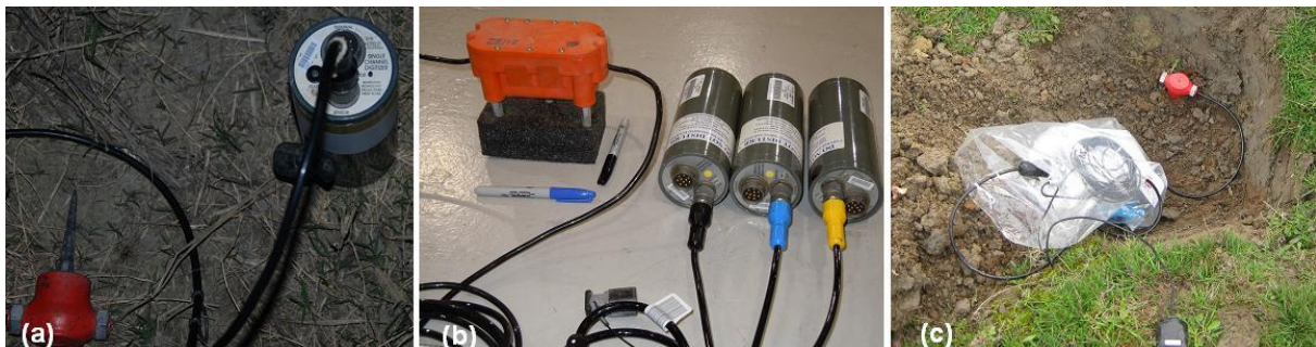
Figure 3.1 (a) photo of “Texan” seismometer attached to a vertical component sensor; (b) Photo of 3 “Texan” seismometers connected to a 3 component sensor (Black – Vertical, Blue – North, Yellow- East; (c) Photo of the ERI “Lunchbox” seismometers connected to a vertical sensor.
