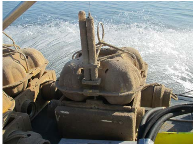
OBS encrusted in barnacles after 1-mos deployment.
