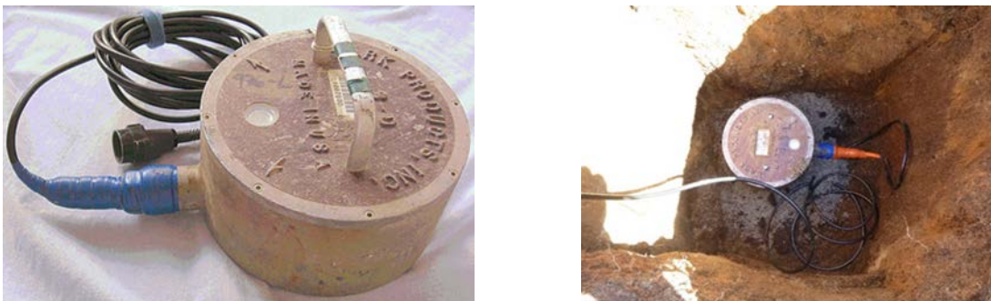
Figure 2.4 The L-22 sensor (left; photo courtesy of PASSCAL instrument centre). L-22 sensor deployed in hole during SHIRE I deployment (right; photo courtesy of Jenny Black).
