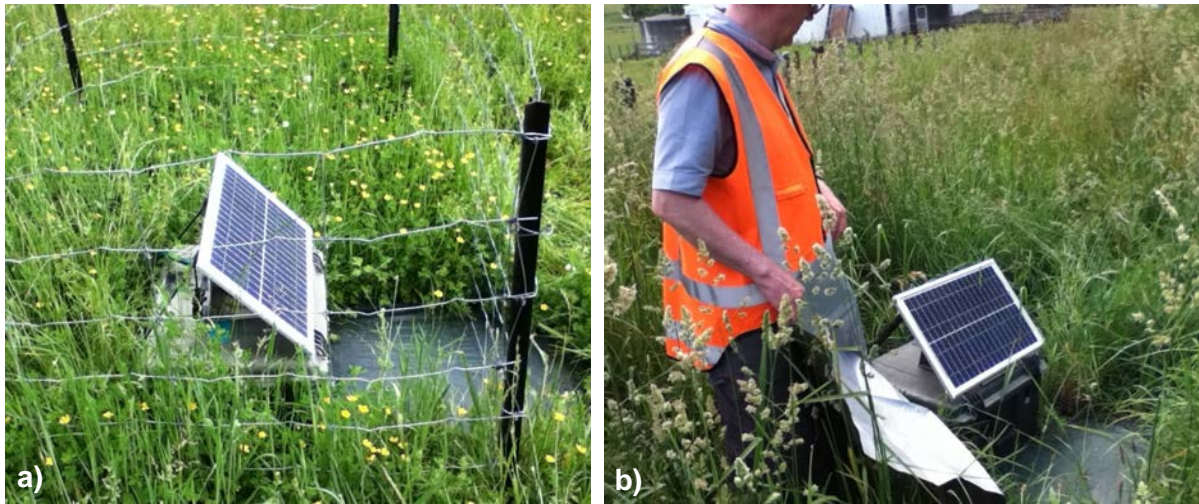
Figure A7.2 Managing vegetation growth at sites. a) Site 716 showing the effects of the tarpaulin to keep vegetation growth down. b) Extreme summer growth at Site 505 required extra tarpaulins.
