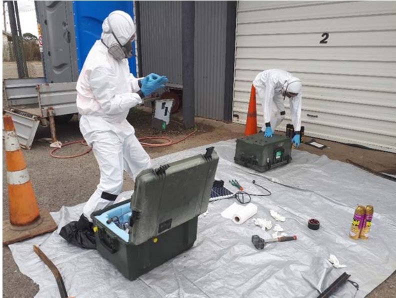
Figure A7.3 Decontaminating the QDS boxes prior to shipping back to PASSCAL. Insects found a home in the QDS boxes during the four-month-long SHIRE I deployment.
