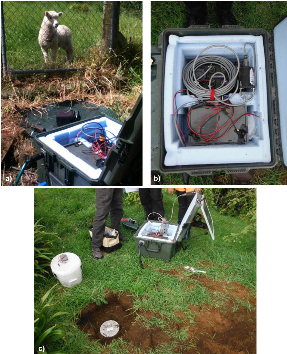
Figure 2.6 Quick deploy station boxes (QDS) in the field. a) Open box showing battery, data logger with connecting cables and small green tarpaulin to limit vegetation growth from blocking the low solar panel. b) Open QDS box shown as configured to leave the site and close the box. c) General site set-up with sensor in foreground, showing solar panel on top of QDS box and cabling buried underground to sensor.
