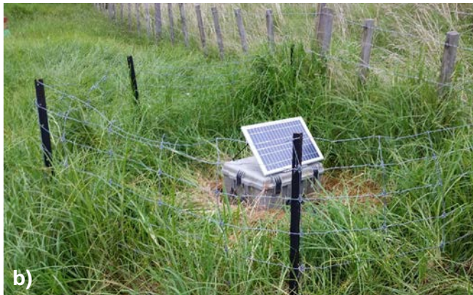
Figure A7.1 Examples of SHIRE site fencing. a) Site 714; waratah enclosure fencing adjoining existing fence and deployment of QDS box. A tarpaulin was used in front of the solar panels and was effective for keeping down vegetation growth. Tarpaulins were not deployed at all sites, and no power loss was attributed to blocked solar panels. b) Site 595; stock have bent the fencing slightly, but it is largely intact. Note how the fencing wire is tucked into the top hook on the waratah to minimise sagging and prevent the wire from sliding down. c) Site 715; isolated fencing enclosure. Extra waratahs and a non-rectangular shape used to increase strength and distance between fence and solar panel.
