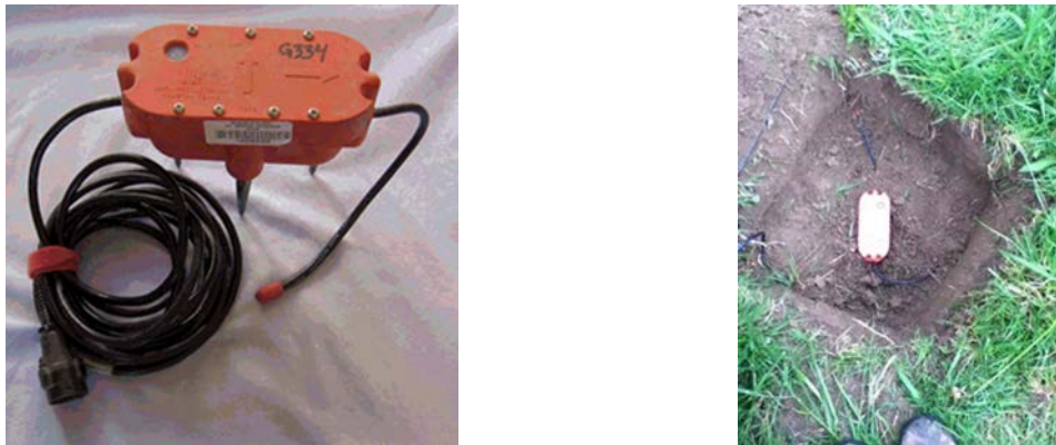
Figure 2.5 The L-28 sensor (left; photo courtesy of PASSCAL Instrument Centre). L-28 sensor installed in a soil site (right; photo courtesy of Pasan Herath).
