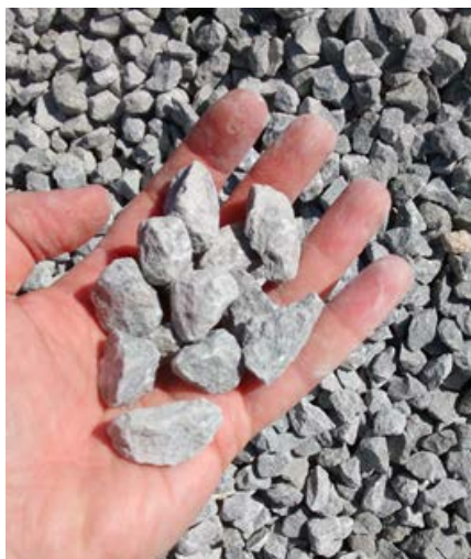
Figure 3.5 Gravels for stemming the explosives in the borehole. 20 mm lime chip used in Sites 1–4.
