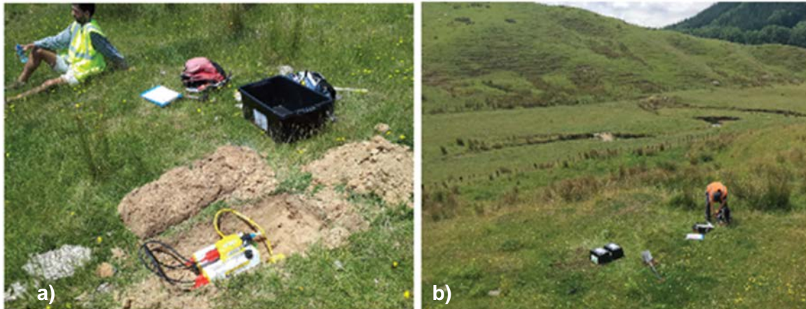
Figure 2.7 Deployment of the GSX3 involved a) digging a ~30-cm-deep hole and stabbing the geophone into the ground. The geophone is then buried (on the right-hand side of the hole), with the two batteries and yellow GSX3 recorder buried to the left of the geophone. b) The area is then covered by two plastic boxes in order to protect it from livestock.
