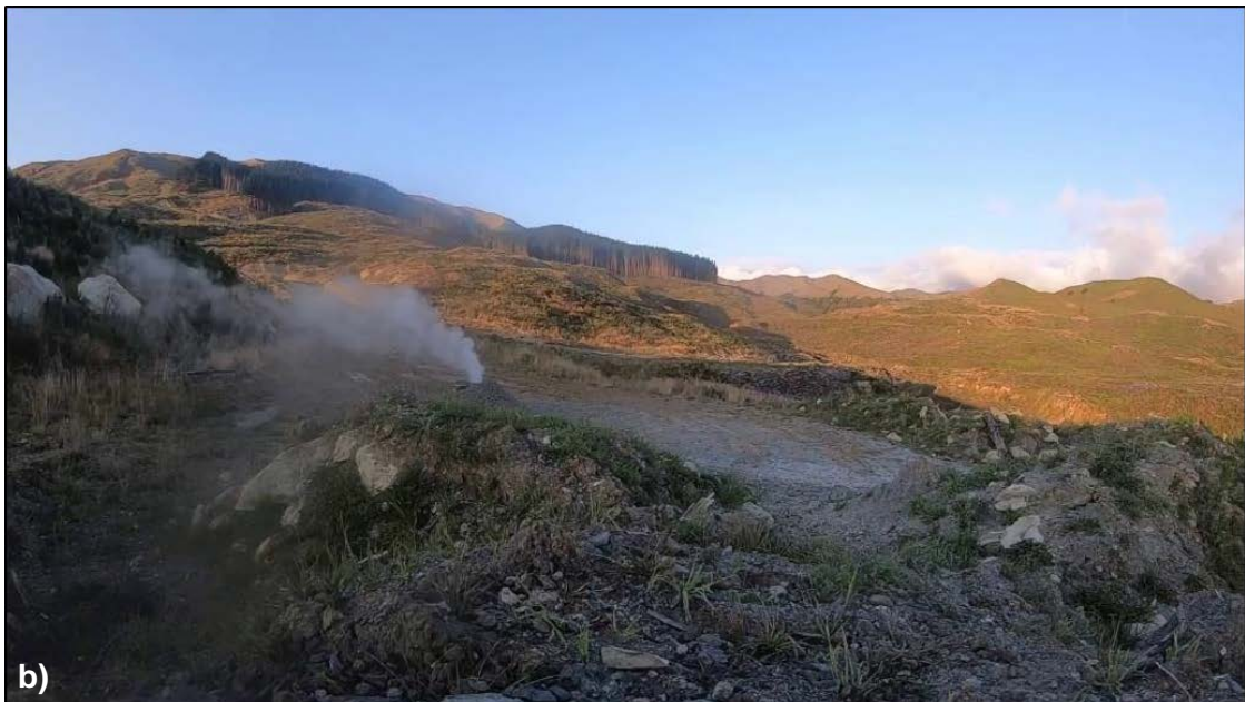
Figure A5.7 Site 3, Blast 2: a) ejection in full progress 55 seconds after detonation and b) degassing at 1 minutes 20 seconds.
