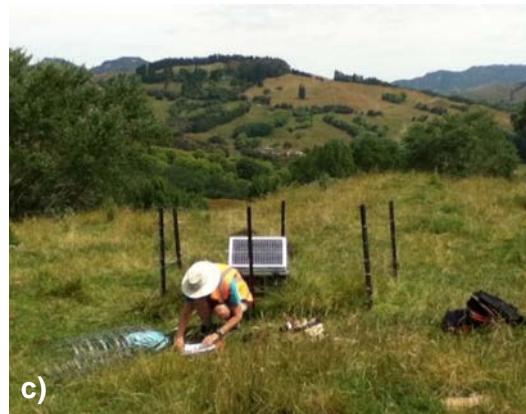
Figure A7.1 Examples of SHIRE site fencing. a) Site 714; waratah enclosure fencing adjoining existing fence and deployment of QDS box. A tarpaulin was used in front of the solar panels and was effective for keeping down vegetation growth. Tarpaulins were not deployed at all sites, and no power loss was attributed to blocked solar panels. b) Site 595; stock have bent the fencing slightly, but it is largely intact. Note how the fencing wire is tucked into the top hook on the waratah to minimise sagging and prevent the wire from sliding down. c) Site 715; isolated fencing enclosure. Extra waratahs and a non-rectangular shape used to increase strength and distance between fence and solar panel.
