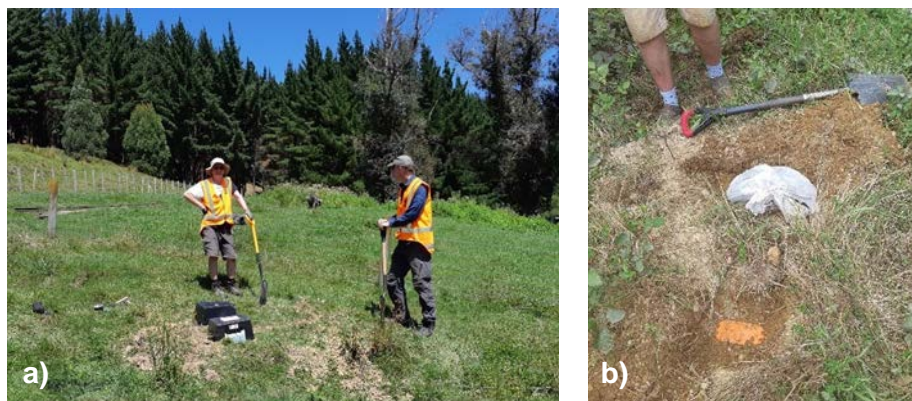
Figure 3.10 a) Example of 2D Array low-profile set-up without fencing. b) 3C Texan site showing separate burial of L-28 and the Texans (inside white bag for extra water and dirt protection). Photos courtesy of Jenny Black.
