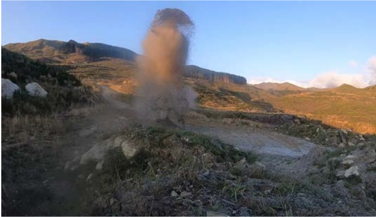
Figure 3.6 Explosion Site 3, Mangatu Forest, detonated 27 February 2019. Venting column of gas and stemming took place approximately 52 seconds after the initial detonation. In the subsequent 10 seconds, the column grew to a height of ~50 m before venting stopped. The image was taken with a Go-Pro camera mounted a few metres from the bore hole.
