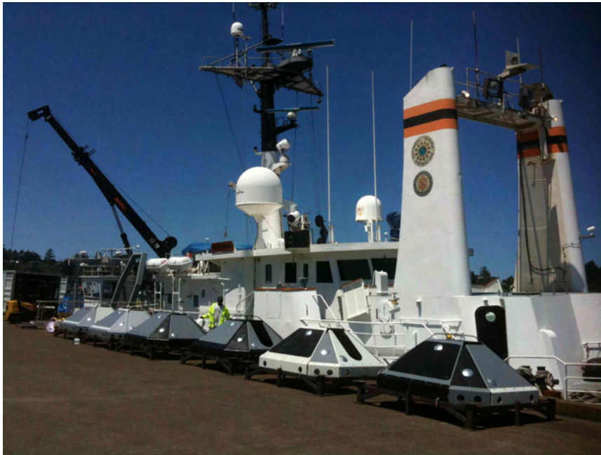
Figure 1: 6 TRM frames on the dock waiting for their final coat of anti-fouling paint before being loaded aboard the R/V Wecoma in Newport, OR. July 23, 2011.
