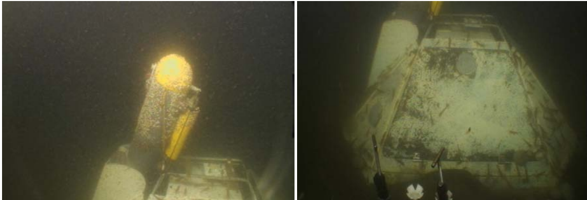
Figure 20. Dive J2-657 at TRM FN01A. The release was covered in barnacles and the safety line securing it the TRM had broken, leaving just the pop-up line hold it to the bail (left). Jason aligned perpendicular to bails at heading of 302 (right).
