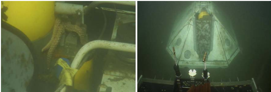
Figure 16. Star-fish blocking the latch release for the pop-up buoy (left). FN07A was oriented parallel to the bails with Jason's heading at 294.
