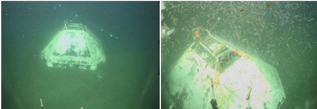
Figure 13. FN14A aligned perpendicular to the bail bars with Jason on a heading of 078 (left). The shackle that had been covered in carpet for release was atop the TRM rather than hanging to the side on its bikini buffer as we'd hoped (right). This site was notable for a large red fish/krill/shrimp swarm!
