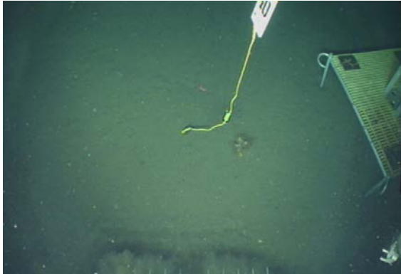
Figure 3. A micro-mooring with a thermistor was deployed for Paul Johnson (UW) to aid in interpretation of data from his thermal blankets being deployed next to two of our TRM sites. We were able to accomplish this ancillary deployment at no time cost to our cruise.
