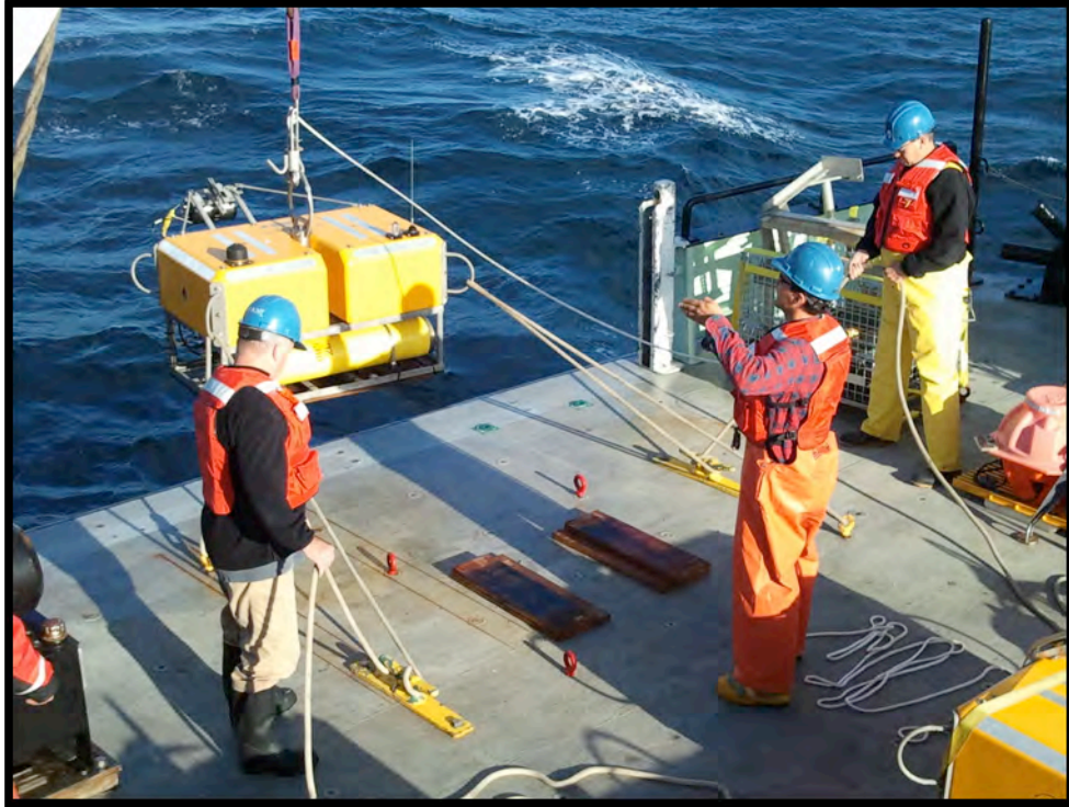
Figure 4. Deploying a WHOI ARRA OBS.
