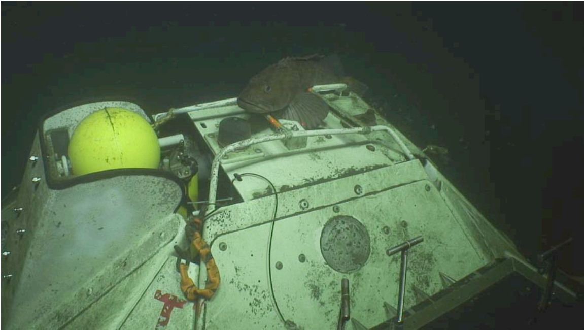
Release mechanism for pop-up float. A little nudge from Jason was all it needed!
