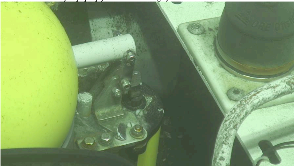
Release mechanism for pop-up float. A little nudge from Jason was all it needed!
