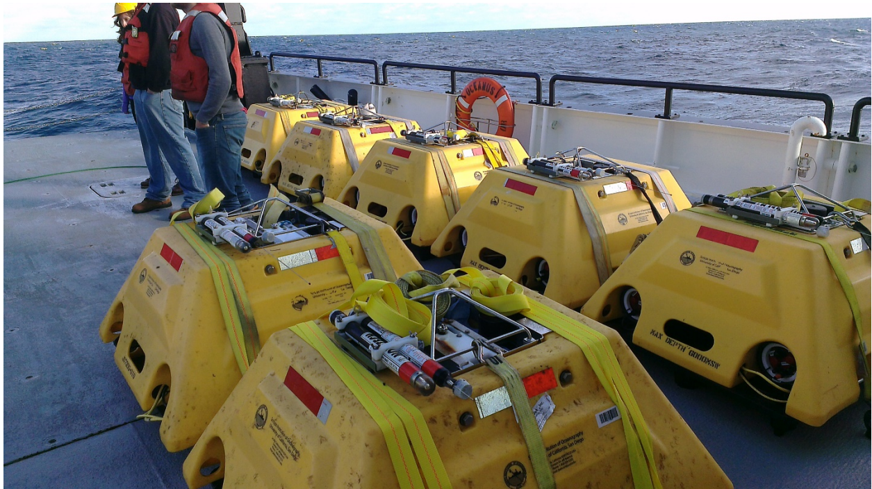
Figure 2. Abalone trawl protected OBS, secured on deck of R/V Oceanus. Recovered after one year deployment.
