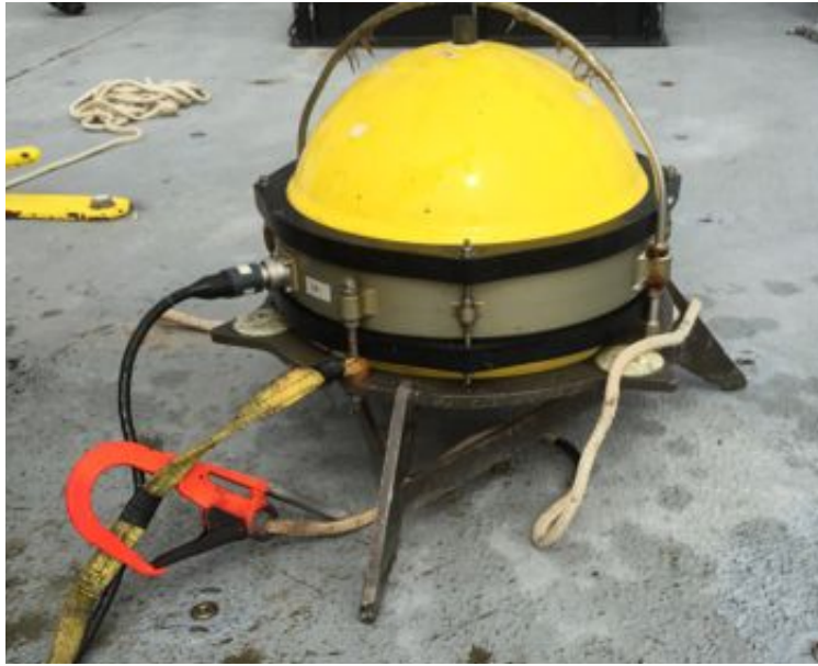
Figure 5. View of the “feet” added to the pressure housing holding the Guralp CMG-3T seismometer. The goal was to improve coupling to ground.
