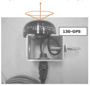
On older 130-GPS units this is indicated by the arrows on the front and back of the unit). Mount the GPS unit with the arrows facing up with an unobstructed overhead view.
