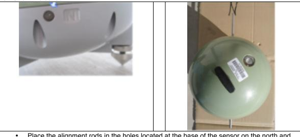
Place the alignment rods in the holes located at the base of the sensor on the north and south sides. Align the rods with the North/South line on the sensor pad. Make sure the bold "**N**" is oriented toward the north direction.
